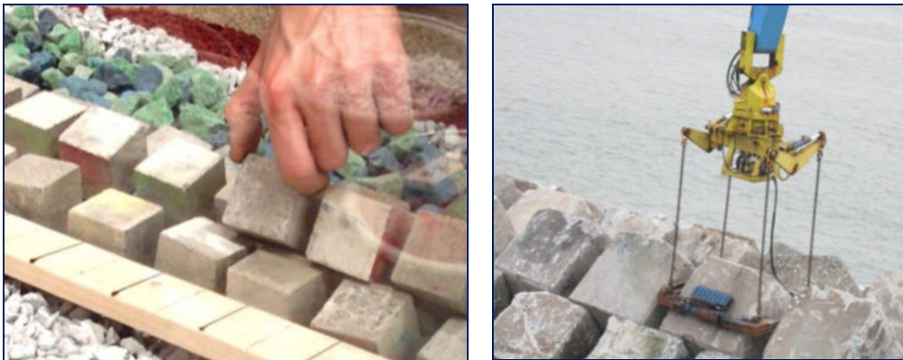
Figure 5. Placement of model cubes according to a protocol that represents reality in prototype.
