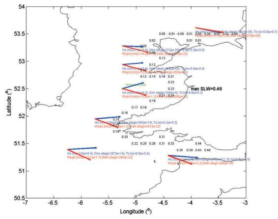
Example of a scenario plot. Mean values (and standard deviations) of the wave parameters (in red), wind parameters (in blue), and water levels (in black and only means) in several locations for when the mean wave direction is between 247°N and 262.5°N the significant wave height is between 2 and 2.5 m and the wind direction is between 187°N and 7.5°N at the reference location (see green).
