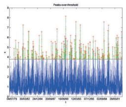
Example of peaks-over-threshold plot. Blue: all values. Green: values higher than the chosen threshold (3.8 m). Red: the maximum values of independent events (more than 48 hours apart
