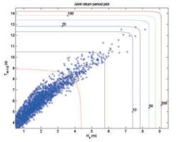
Example of a joint return value plot of significant wave height (Hs) and mean wave period (Tm-1,0).
