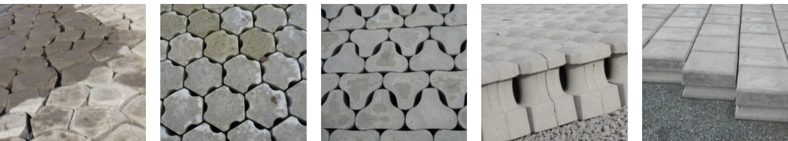
Figure 2 Different types of block revetments tested (from left to right: Basalton ® , RONA ® ton, C-Star ® , Hillblock ® , Verkalit ® )
