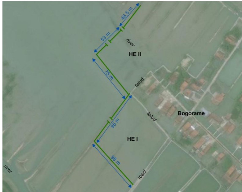
Figure 21 Design of two permeable structure grids at the coastline of Bogorame.
