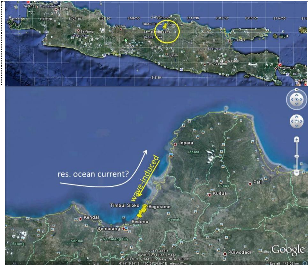
Figure 4: Java with Demak coast indicated by yellow circle (upper panel) and close-up of Demak district and coastline (lower panel), including indications of residual sediment transport.
