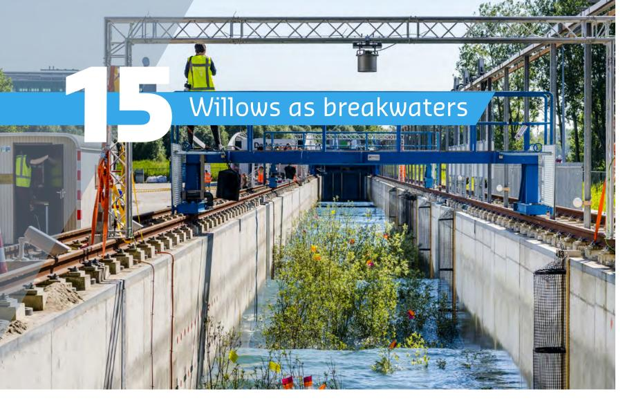
Vegetation has the potential to reduce the wave load on many kilometres of dike in the Dutch river area. That potential has not yet been fully mapped out, in part because of knowledge gaps in the area of wave mitigation with vegetation.
