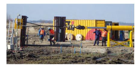
deformation behaviour and the strength of this kind of dike. A few weeks earlier, a dike without sheet piling had already been collapsed. Comparing the two made it possible to identify differences between dikes with and without sheet piling. Continuous monitoring took place during the trial to establish a range of datasets.
