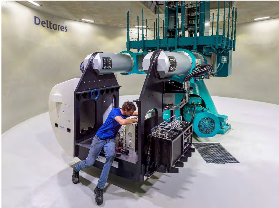
Figure 7.5: Deltares GeoCentrifuge setting up an experiment.
