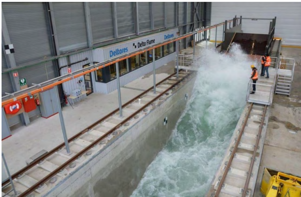
Figure 7.6: Deltares Delta Flume experiment.
