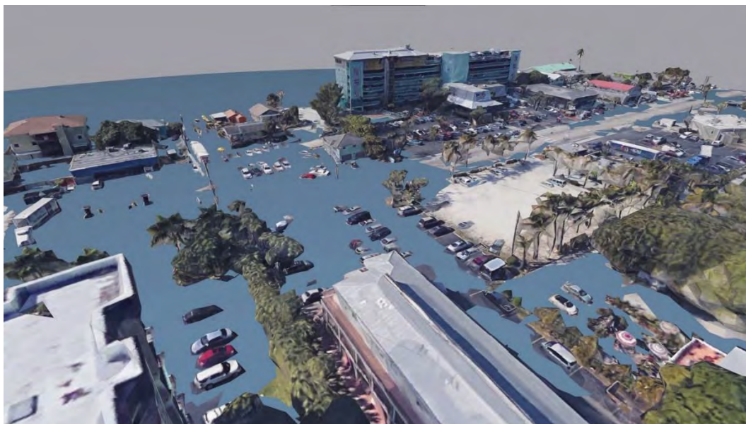
Figure 3.2: Still photograph of an XBeach simulation of flooding in Ft. Meyers Beach due to Hurricane Ian (September 2022).
