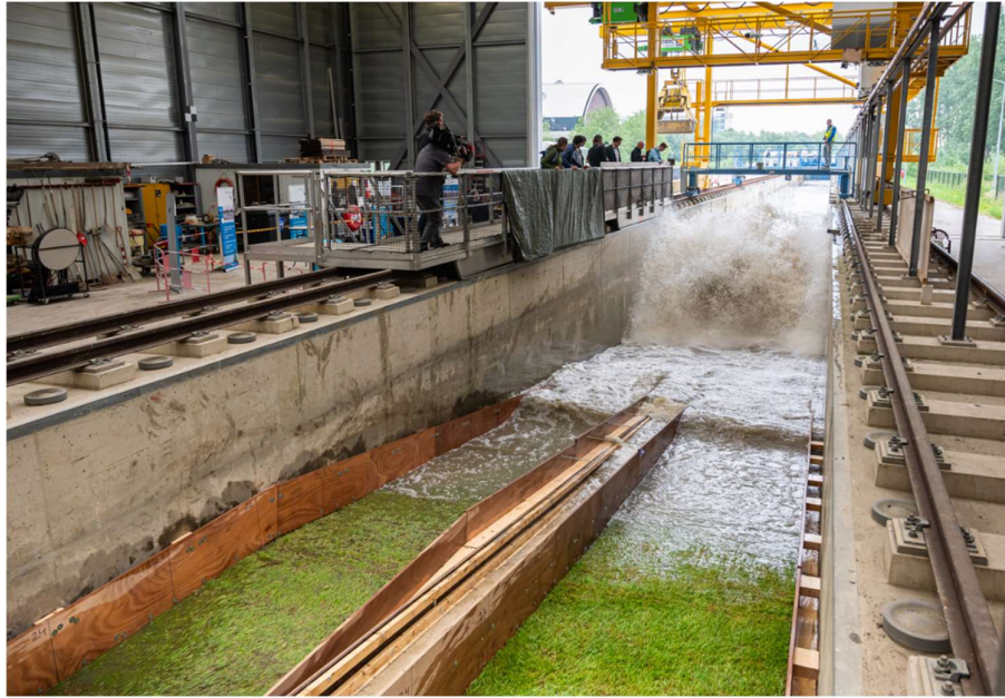
Figure 3.3: Impression of research on erosion of grass revetments with underlayer of clay under wave loading in the Deltares Delta Flume. Obtained empirical data will be combined with physical understanding, numerical modelling and integrated into a toolbox that be used to quantify the failure probability of revetments including underlayers of clay.
