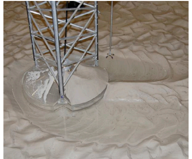
Scour at model of jack-up foundation
