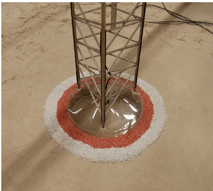
Transparent model equipped with a high-resolution camera and scour protection
