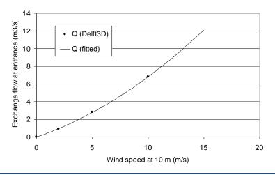
Figure 4.9 Wind-induced exchange flow Q in the harbour mouth  $(m^3/s)$  as a function of the wind speed W at 10 m (m/s). Results from Delft3D numerical experiments and a line fitted through these results ( $Q = 0.0255 W^2 + 0.4257 W$ ).
