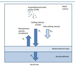
Figure 6.2 Schematic overview of vertical fluxes in a water-sediment column.
