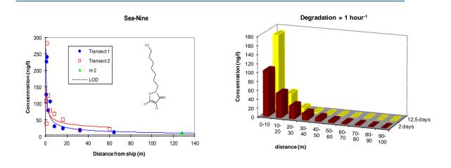
Figure 7.2 Observed (left panel) and predicted concentrations (ng/L) of DCOIT (Sea-Nine<sup>TM</sup>) in the Korsør harbour study with two freshly painted naval ships. Observed concentrations: adapted from Steen et al. (2004). Predicted concentrations: simulations with MAMPEC v2.0, settings based on data in Steen et al. (2004)
