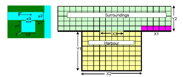
The PEC profile outside the harbour is shown for the area indicated by the pink grid cells in the picture above: the cells downstream of the harbour on the harbour side of the river. The profile gives an indication of the dilution in the surroundings.
