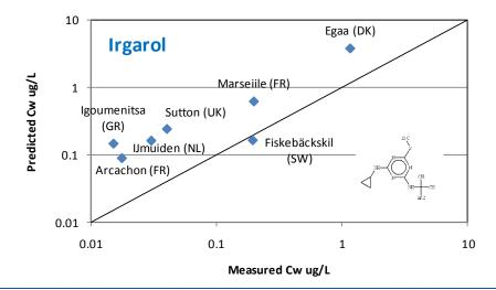
Figure 7.1 Comparison of measured concentrations of Irgarol (µg/L; average values) in European marinas and predictions (average concentrations) derived with MAMPEC v 3.0. Source measured concentrations: Readman (2002). MAMPEC scenarios: van Hattum et al. (2002).
