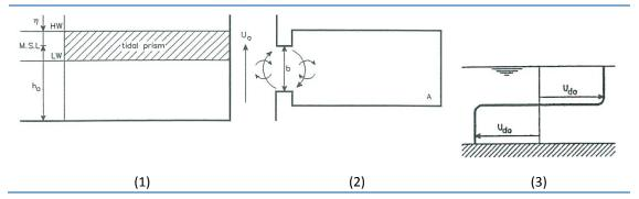
Figure 4.1 Main phenomena responsible for the exchange of water in harbours: (1) tidal exchange, (2) horizontal exchange, (3) density driven exchange
