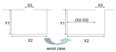
Figure 4.13 Schematic representation of a harbour with a small entrance
