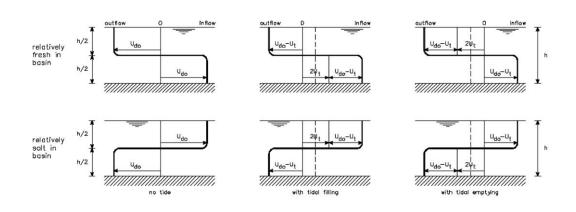
Figure 4.2 Schematized flow profiles indicating reduction of density induced exchange flow by tidal filling or emptying of basin.
