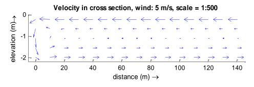
Figure 4.7 Flow velocity in harbour – cross sectional view, open boundary is on the right; 5 m/s
