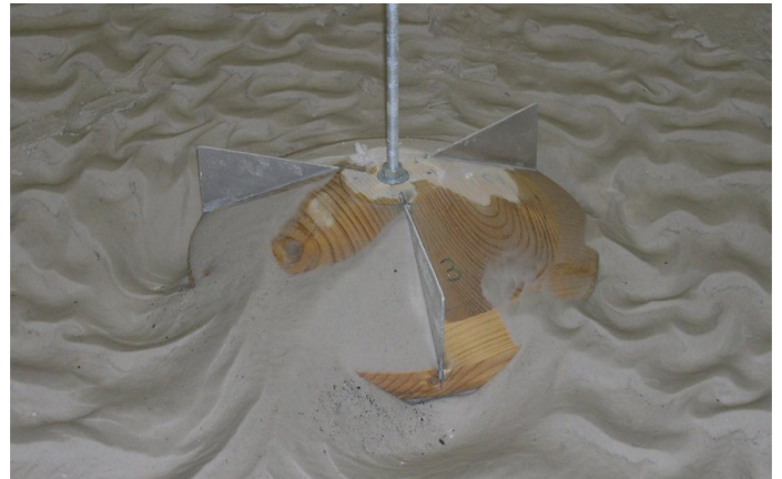
Example of physical model test with similar scour pattern
