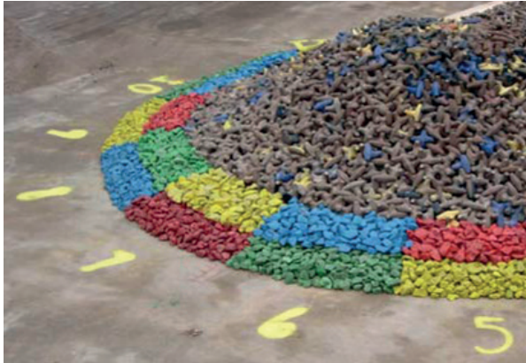
Testing the stability of a breakwater roundhead
