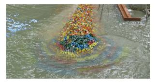
Testing a breakwater model and studying the wave climate
