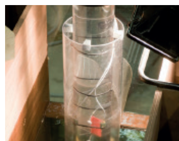
Pump model in pump compartment
