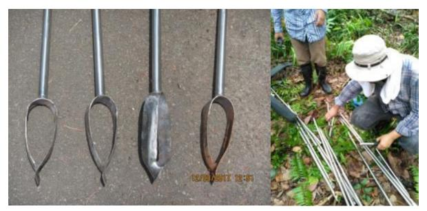
**Figure 37** (LEFT) Edelman type auger heads used in this peat survey. (RIGHT) team preparing the auger at the survey location.
