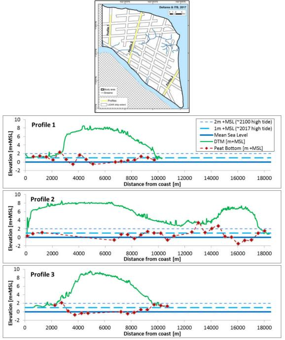
**Figure 12** Three cross sections over the two Bengkalis Island peat domes along LiDAR flight lines, showing LiDAR derived surface elevation (DTM) and the peat bottom as derived from field measurements. The North side is on the left in all profiles. Mean Sea level and estimated likely High Tide levels are also shown. *Note:*
