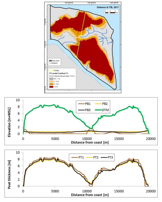
**Figure 24** Cross section through the two Bengkalis peat domes showing LiDAR based peat surface elevation (DTM), peat thickness and peat bottom elevation according to 3 peat models. For methods see caption in Figure 22.
