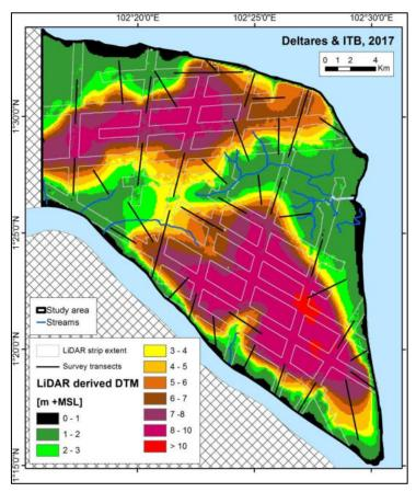
**Figure 6** Peat thickness survey design along 44 transects, starting at areas where no peat was expected going perpendicular up the dome. In the background DTM generated from the LiDAR strip data (Figure 8).
