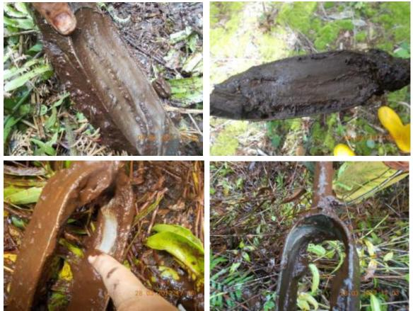
Figure A.5 The example of auger that has reached the mineral soil (clay).
