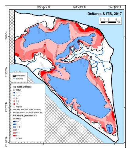
**Figure 19** Peat bottom model as derived from subtracting actual field peat thickness measurements (Figure 13; black dots) and the LiDAR based DTM (Figure 8); the 0 m +MSL contour lines are added manually between measurements. The peat bottom map is created through inverse distance interpolation between peat bottom measurements, the 0 m +MSL contour lines and the likely maximum peat extent boundary.
