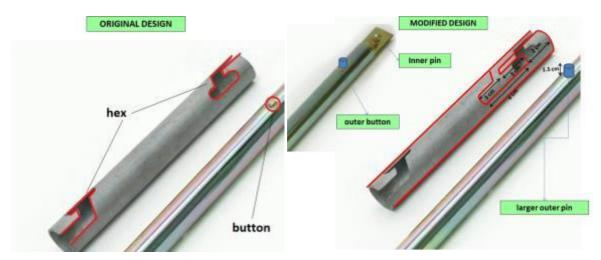
**Figure 39** (LEFT) Original design (RIGHT) Modified design of connector used in the study after several auger heads were lost at the beginning of the survey.
