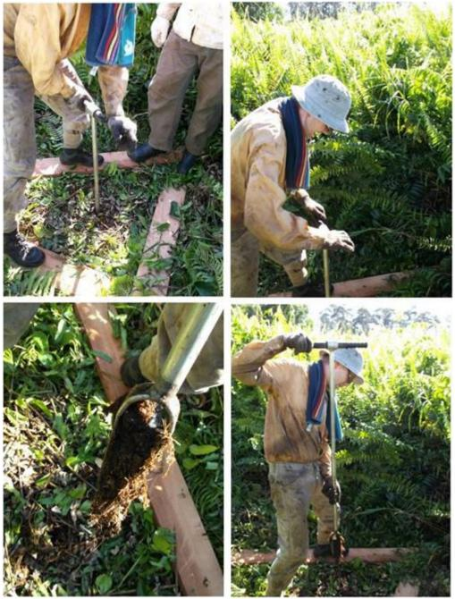
Figure A.2 The initial stage of peat drilling
