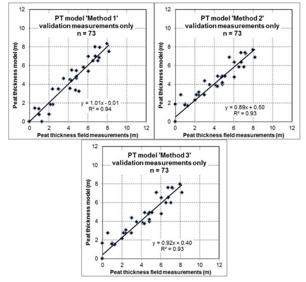
**Figure 23** Modelled peat thickness plotted against peat thickness measurements (the 'validation' dataset (Figure 13) for the 3 different peat thickness models.
