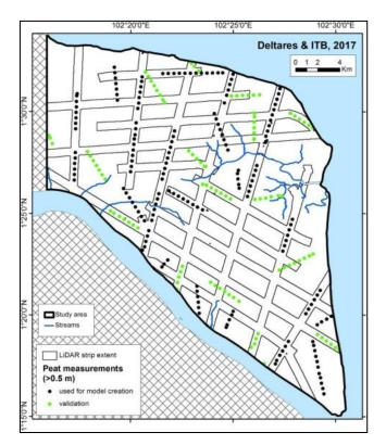
**Figure 13** Distinction between peat thickness measurements in the study area (Figure 10) used further in peat thickness model creation (black dots) and as used for validation. Also shown is the extent of the LiDAR strip data (Figure 8).
