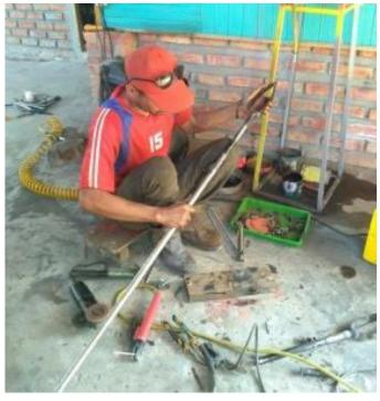
Figure 41 Duplicating auger head in the local workshop.
