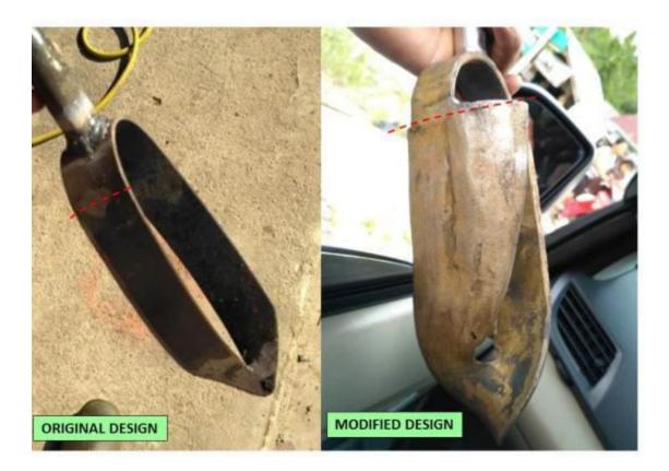
**Figure 40** (LEFT) Original Edelman type auger head used at the start of the survey and (RIGHT) Modified Edelman auger head from week 2 of the survey onwards.
