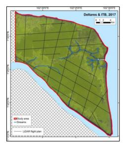
**Figure 4** LiDAR flight plan over IPP study area as designed using existing peat extent maps, historical Landsat imagery (using vegetation patterns indicating presence of peat) and location of rivers and coast. In the background the RGB composite Landsat-1 image of 5 October 1972 (spectral bands 6-7-5) used. LiDAR flight line spacing is mostly at 2.5 km in this study.
