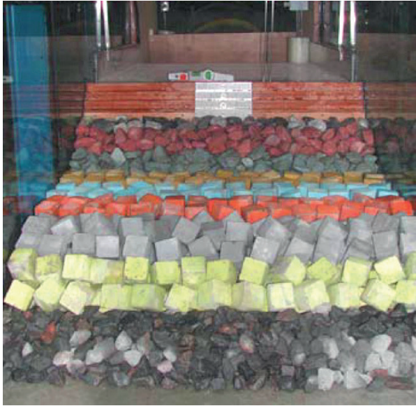
A breakwater model with crest wall in the Scheldt Flume
