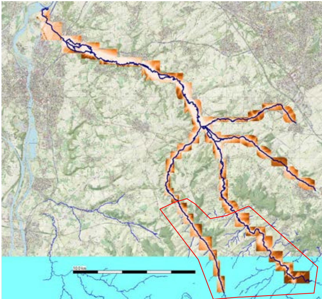
Figure 6.1 Extent of the Sobek2 model of the Geul, including the existing Dutch and (within the red polygon) the new Belgian part. The dark blue lines represent the 1D component of the hydrodynamic model, the brown areas are the DEMs of the 2D component.
