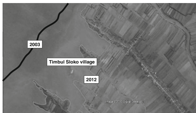
Fig. 2 Coastline changes in Demak District (Timbul Sloko village, Central Java, just east of Semarang) between 2003 and 2012 estimated land loss 200 – 900 m (source: Google Earth )
