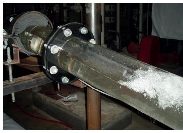
Hydraulic jump demonstrated in a transparent pipe sections
