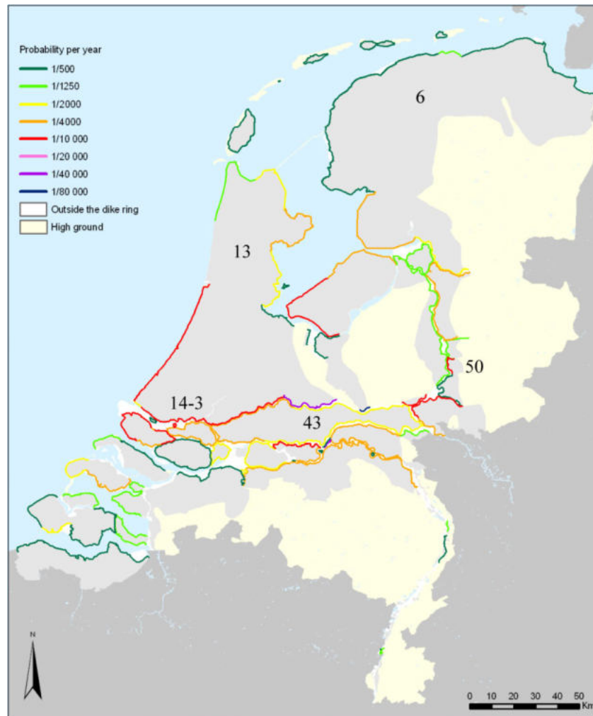
Figure 6 Economically efficient flood protection standards for the Netherlands according to the base scenario. The standards are presented in safety classes (1/2000, 1/4000 etc.), with the boundaries between the classes calculated on a logarithmic scale. For example, the boundary between 1/2000 and 1/4000 is equal to 1/2800 per year [ \approx 10^{(\log(1/2000) + \log(1/4000))/2} ].
