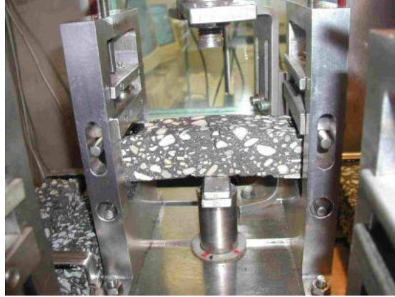
Figure 3. three point bending test, start of yielding
