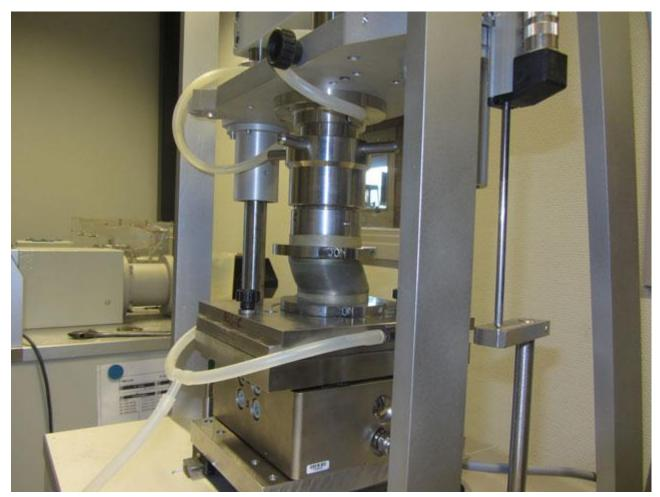
DSS-test part of determination of strength and behaviour of the peat in the new designing method
